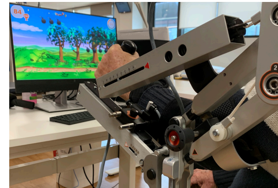
Rehabilitation patient Robert Wells using Armeo Spring:- upper arm rehabilitation robot
